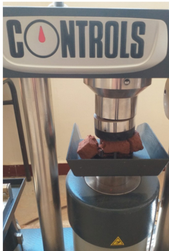
Figure 2 Compressive strength experimental testing set up [37]
