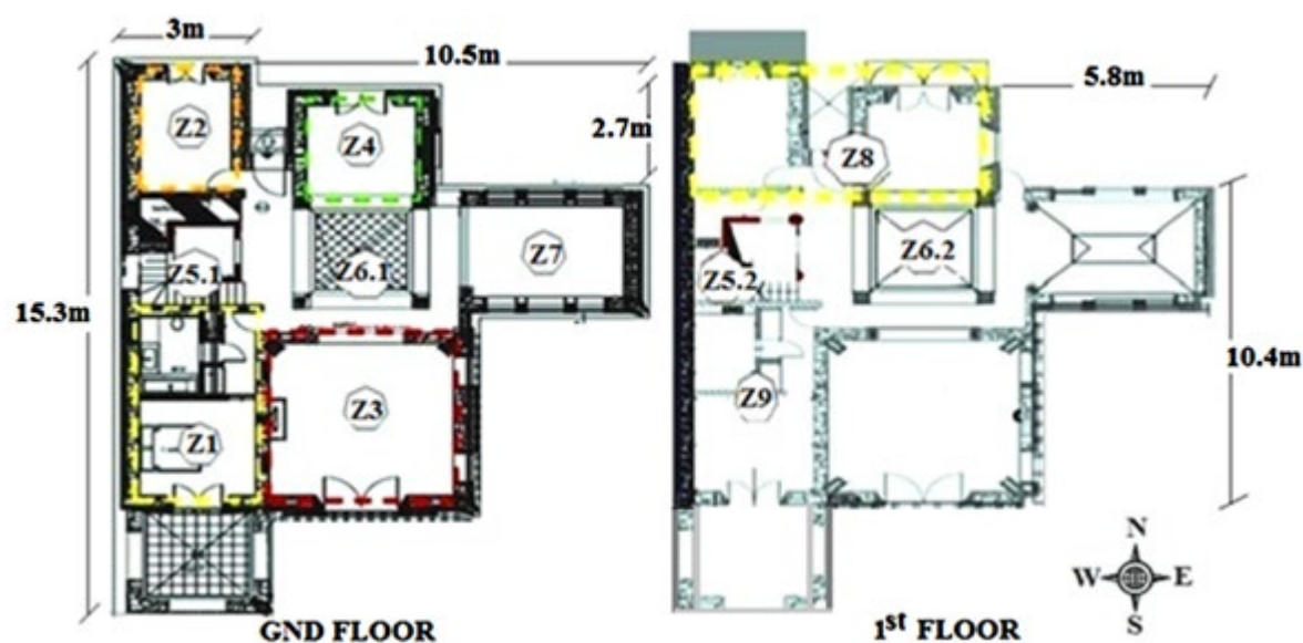
Figure 141 : Architectural plans of the studied house. The thermal zones as defined in TRNSYS are indicated [2].
