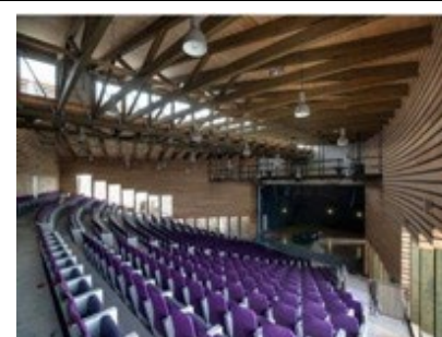
Figure 103: T5 light bulbs (density: 8.7 W/m 2 )
