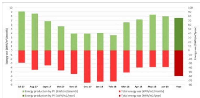
Figure 16: Monthly and yearly energy production by PV (green) and total energy use (red) during the investigated year (2017/2018)
