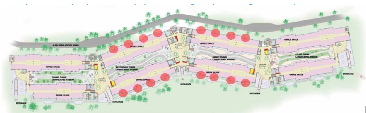
Figure 3. With red dots, the office locations liable to glare for lack of shading devices are here shown.
