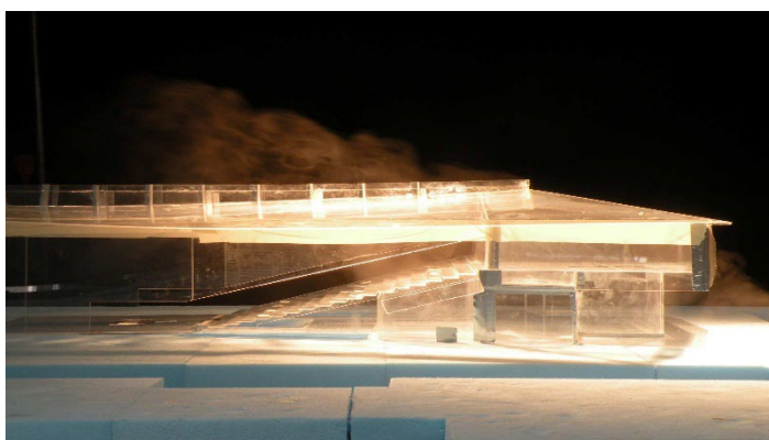
Figure 96 : Wind tunnel tests to validate the passive principles
