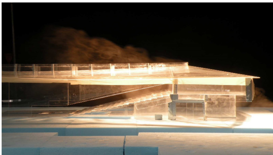
Figure 15 Wind tunnel tests carried out to validate the natural ventilation strategy set up for the Moufia bioclimatic theatre, in La Reunion.
