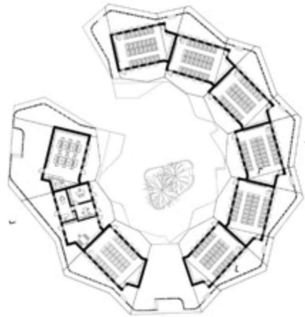
Figure 94 : Floor plan of the Lycée Schorge. The modular structures are arranged radially around a courtyard. © Kéré Architecture
