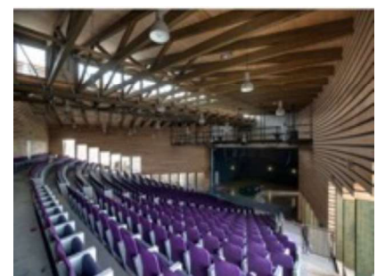
Figure 103: T5 light bulbs (density: 8.7 W/m 2 )
