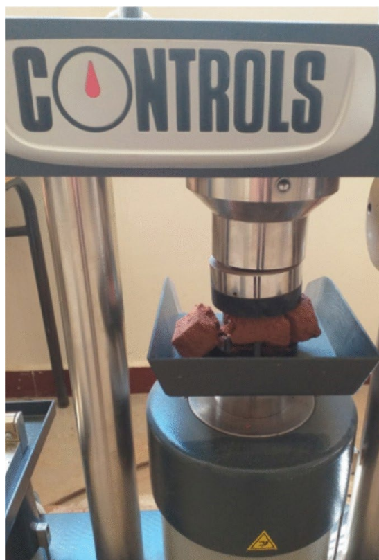
Figure 2 Compressive strength experimental testing set up via CONTROLS machine [37]
