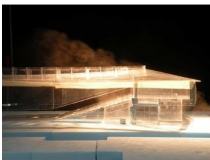
Figure 98 : Wind tunnel tests to validate the passive principles
